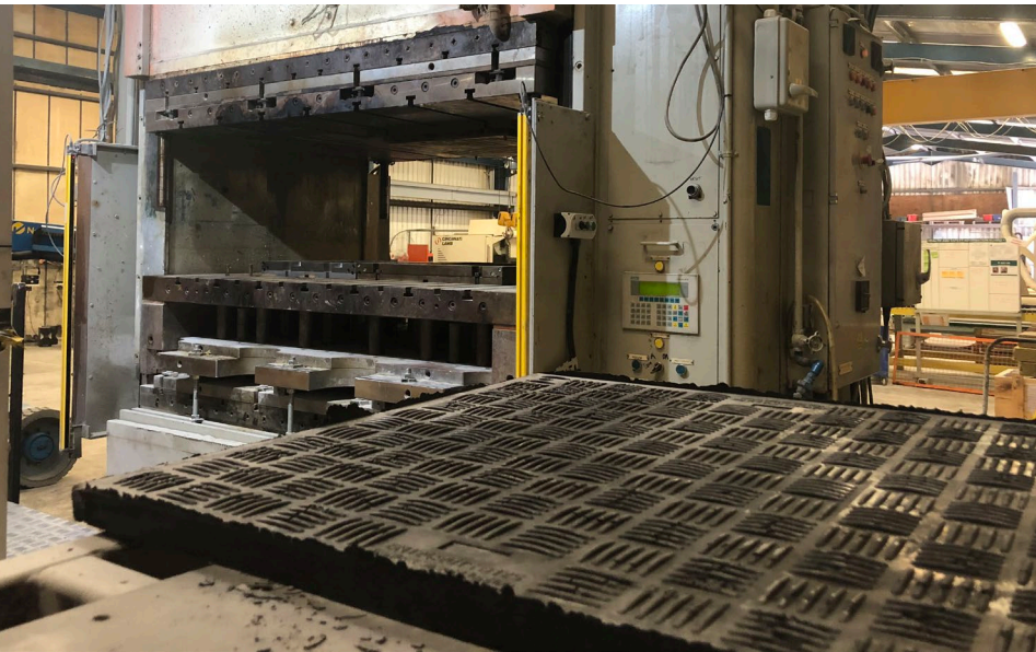
Pultrusion of Handrails & Compression moulding of manhole covers, both in Glass Fibre Reinforced Polyester Resin type composite materials.
