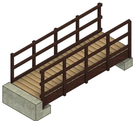
Existing abutments can be used. They may not always be concrete. Soil may need to be retained
