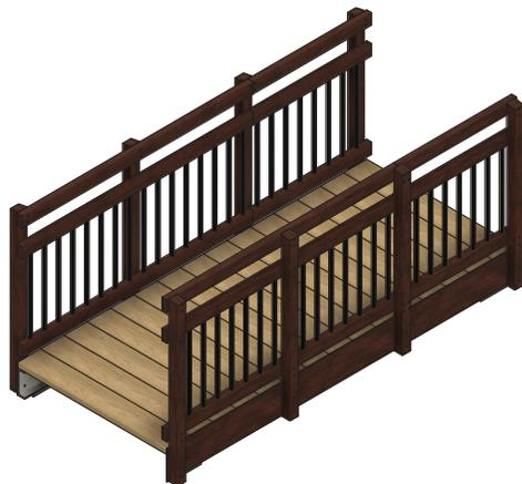
Infill panels. Utilising POLYbridge rails and pultruded GRP infill tubes.
