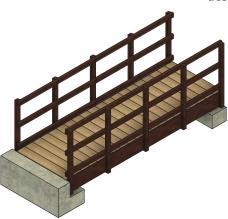
Existing abutments can be used. They may not always be concrete. Soil may need to be retained
